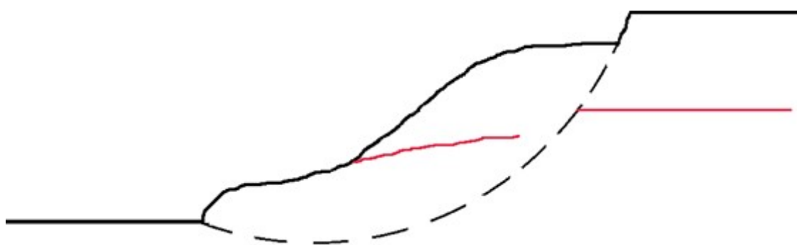
Breaking of reinforcement - type of failure 1
