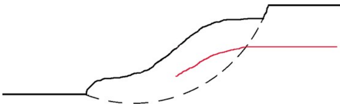
Pullout of the reinforcement in front of the slip surface - type of failure 3
