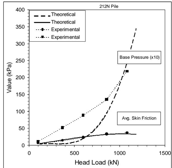
Figure 11. Comparative Results for the 212N Pile.
