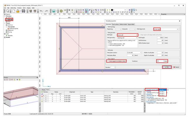
We add the walls graphically by using the mouse, click on the points of intersection bewteen the walls and the construction lines. Watch out for the input direction, the wall alignment meets "to the right".
