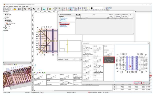
Before we go on, we thoroughly check the model if it satisfies all input and other criteria, if no trusses are missing, no collisions occur, etc.
