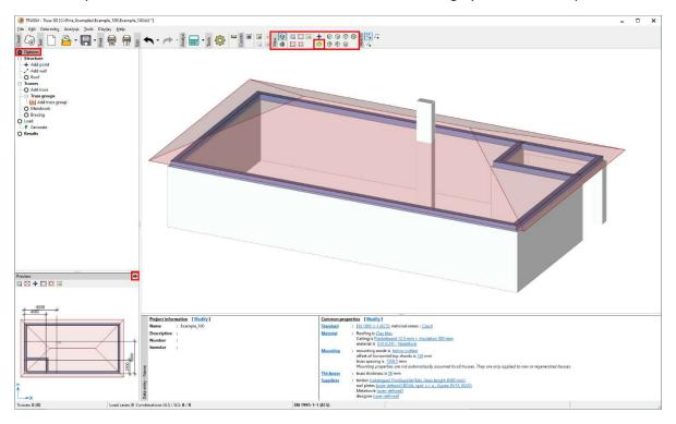
We delete the construction lines as we won't need them anymore. First, we switch back to plan view, then hit the <ESC> key in order to deselect eventually previously selected objects, then left click on the drawn lines and dimension lines so they get highlighted with green colour and finally hit the <Del> key to delete the selected elements.
