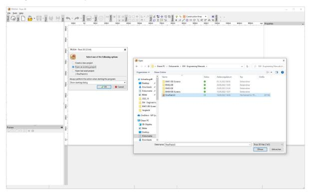
By opening the file "FineTrial.tr3" we received the required catalogues and now can create a new project via the symbol "New".
