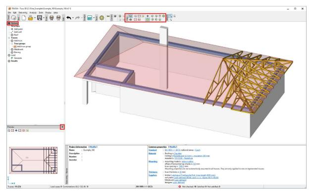
We create the other hip group in a similar way. We click on the walls in this sequence: front roof surface (right -1), side roof surface (upper -2) and side roof surface (lower -3). We end the input of the first phase with a click on "Next".
