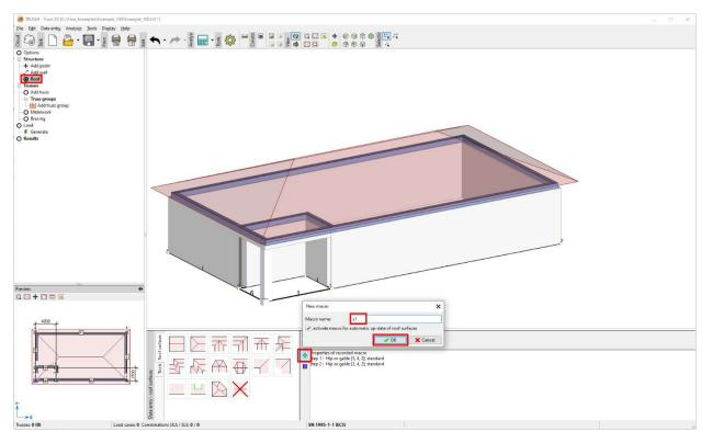
Further we add a chimney using construction lines and parallels. We add a point where those lines intersect and assign it the properties of a chimney.
