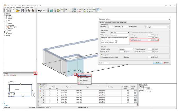
In the same way we change the properties of the edge point to create a column (again this has no impact on design and analysis).
