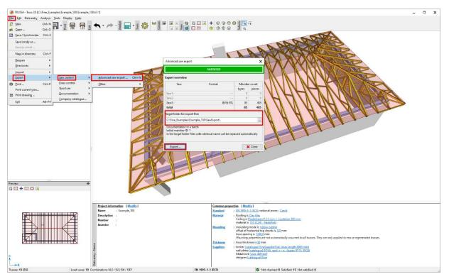
Furthermore, export types are available to other 3rd party programs, such as Dietrichs, Sema, AutoCAD, CADWORK, BIM in the formats of FTD, 3DS, DXF, IFC.
