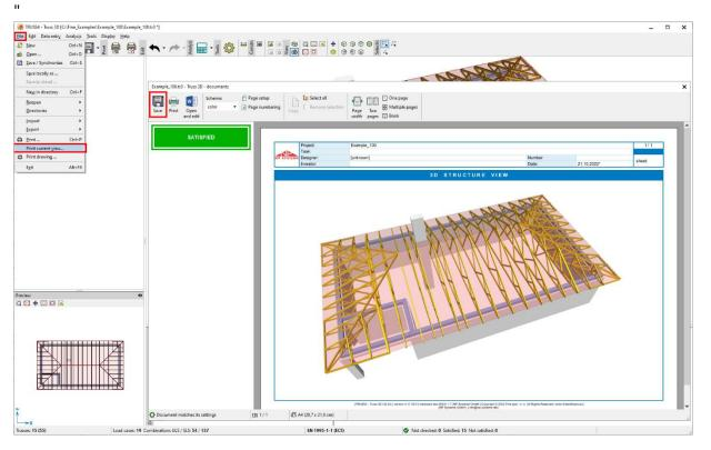
Printing the layout drawing is done via "Drawings...", the user can control the display of elements and dimension lines.
