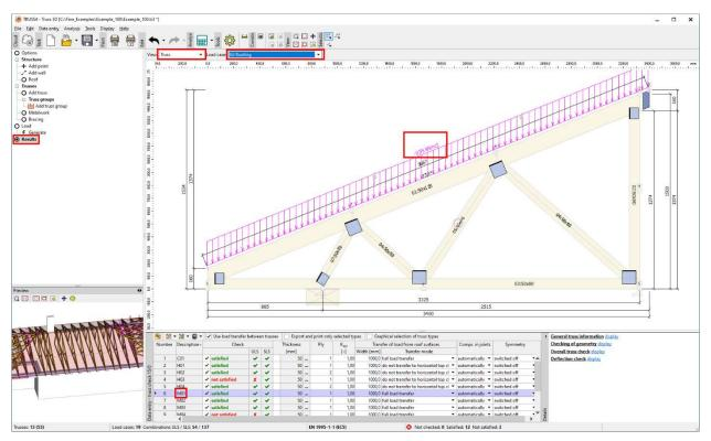
The selection "Truss" enables the display of the loads acting on the truss in the selected load case.
