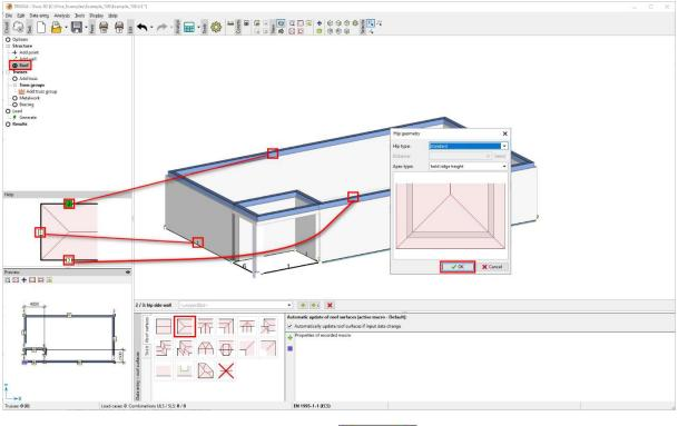
Repeat this for the other hip. Select "hip or gable" And click on the wall on the opposite side of the building again in the sequence hip gable wall (1), hip side wall (2) and hip side wall (3).
