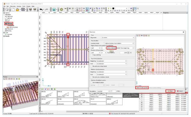
In this second input phase we choose "Truss from structure" and click on the existing truss T01 (select either from table or plan preview)
