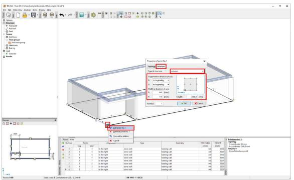
The next step happens in the options window in section "Structure" and the item "Roof". Here you create roof planes. By clicking on "+" you run the roof plane editor.
