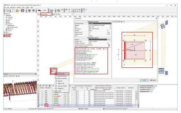
In the given case the compressive stress in the joint line is decisive, which we solve by increasing the cross section of the top chord. We perform this by editing the member's topology on the tab "Section", see picture below.
