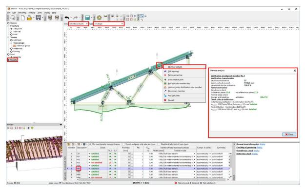
The view "Joint results" displays the utilisation of the joints for the envelope or individual load combinations. Double clicking on the nail plate or the selection via the context menu opens the plate editor in which the plate can be moved, rotated and changed in size and its orientation adjusted. Above that it contains the detailed analysis results.
