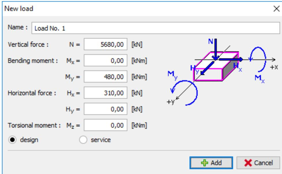
*“New load” Dialog window – Design (calculation) load*
