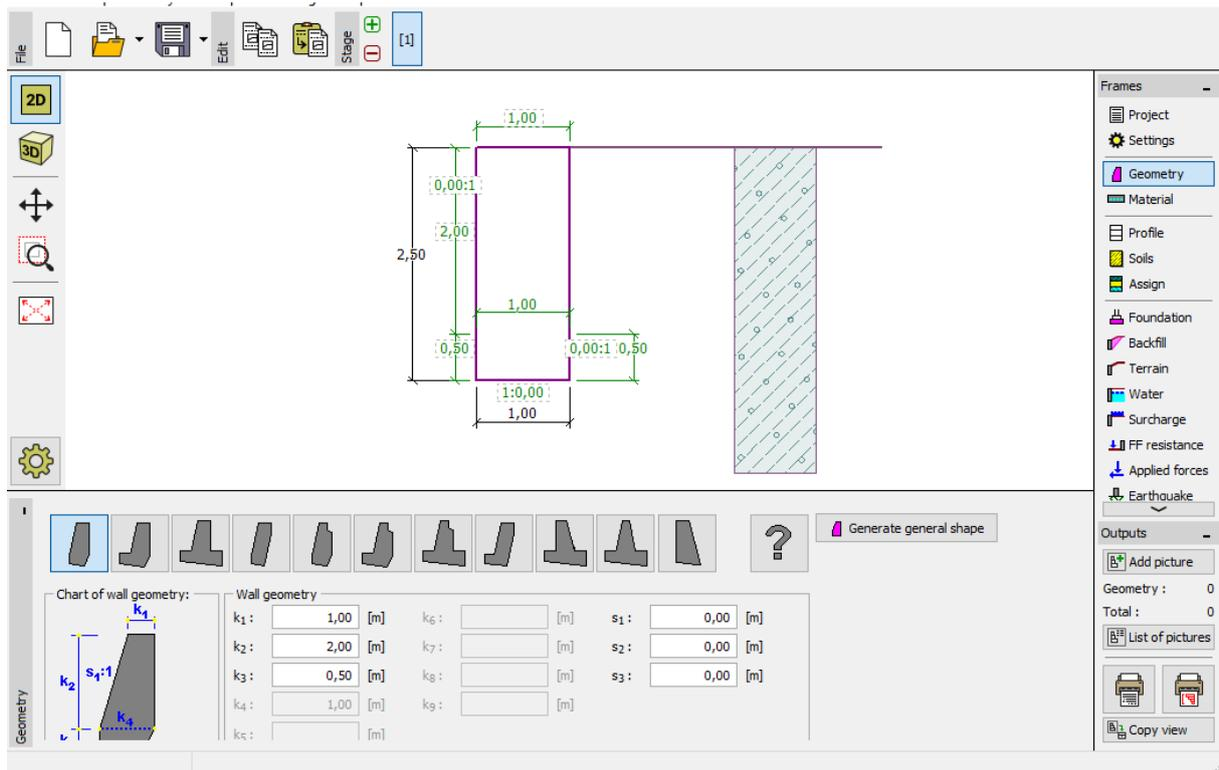
*“Geometry” Frame – gravity wall dimensions input*
