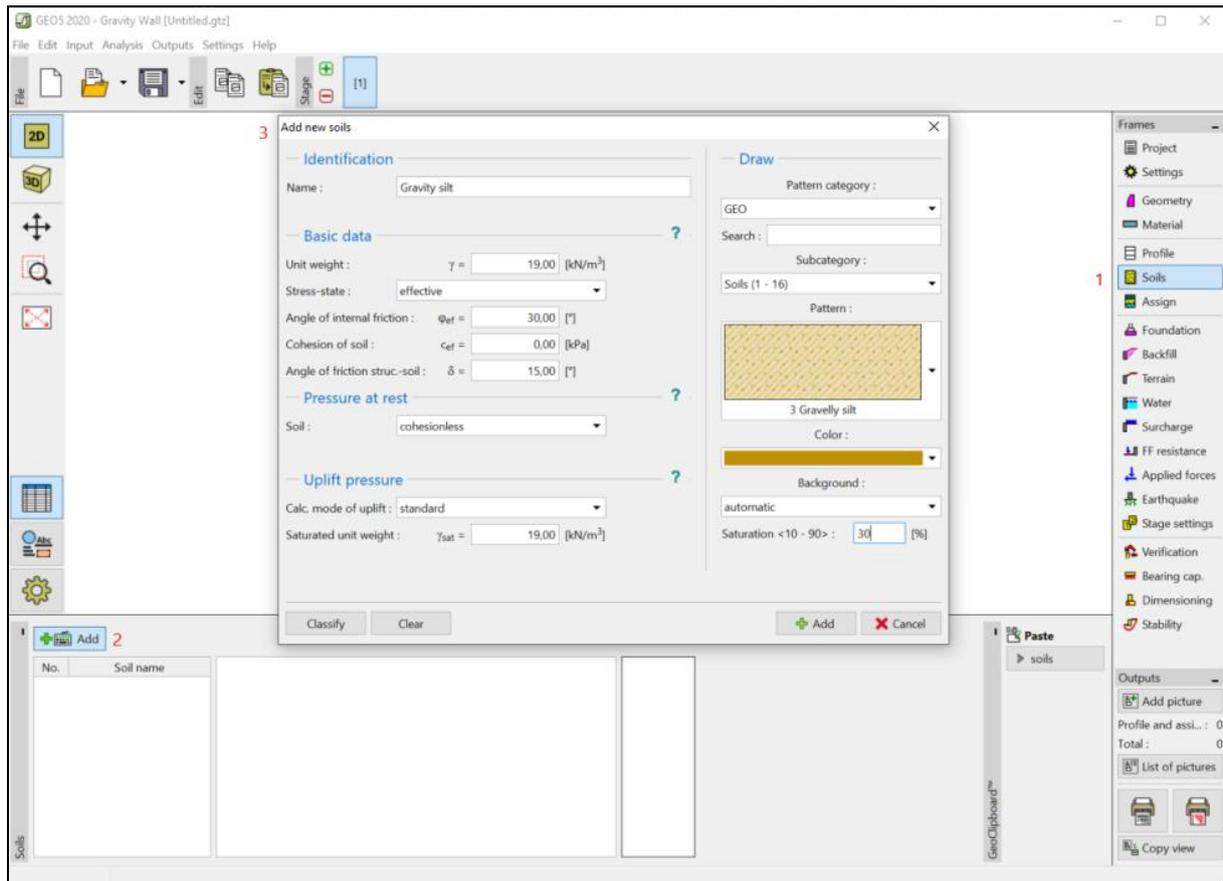
In the “Assign” frame, the first soil will be assigned automatically to the layers. After finishing the basic input of the construction, we can choose the standards we want to use, and then finally run the analysis of the gravity wall.
