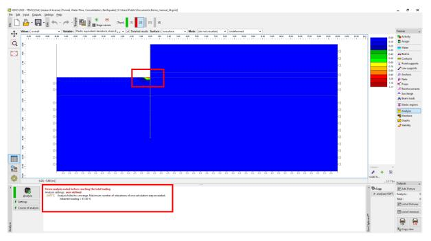
Diverging analysis in the 2<sup>nd</sup> calculation stage
