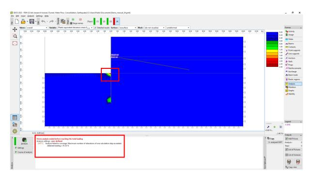
*Equilibrium for the total load not reached in the* 4<sup>th</sup> *calculation stage – no redistribution of plastic strains takes place, analysis is diverging*
