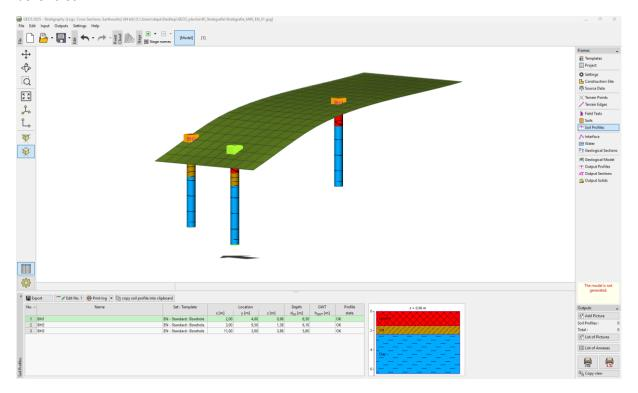
Note: The reason for the existence of Soil profiles is similar to that of "Soils". Complex and detailed boreholes need to be simplified for the geotechnical model. Penetration tests (CPT, SPT) can be interpreted into geological profiles too. This can be done either in this frame or when making geological sections. Creation of earth profiles from field tests is described in EM number 43 – Creation of Soil profiles from Field tests.
