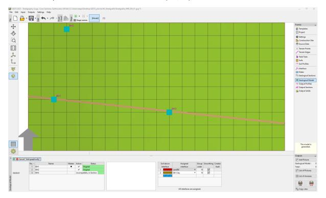
The borehole will be created according to the existing subsoil model.
