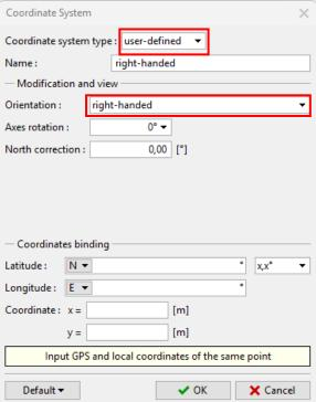
Note: For real constructions, the coordinate system used in the given country or region is selected. In the Czech Republic, it is the JTSK and all coordinates are then added into this coordinate system.
