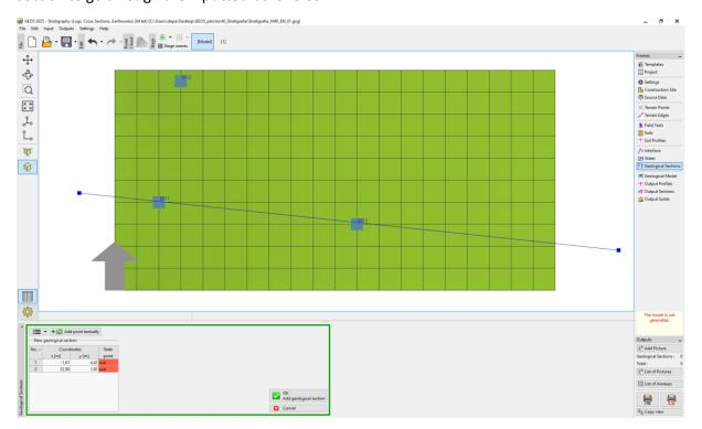
After input, the cross-section is cut into the dimensions of the construction site and opened in the dialog window for edit – in the "Topology" tab. Here, we assign tests that we want to display in the cross-section.
