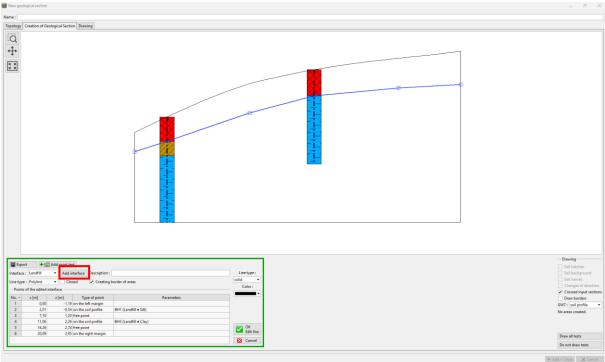
We will define the interface between silt and clay the same way. Do not forget to create a new interface "Silt - Clay"
