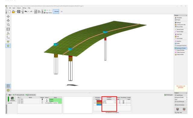
Note: Master borehole must contain all soils (or soil layers), that are present in the model - even those that are not physically in the area of this borehole. This is common when we create a model with lens or faults. For more information, view EM 41– Advanced Modeling in the Stratigraphy Program.
