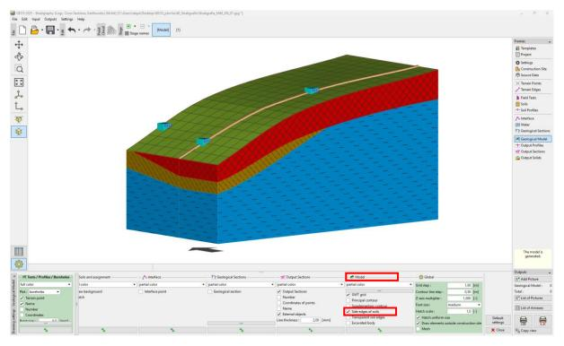
The created model of the subsoil can be further modified using new boreholes. For example, we assume that the landfill layer on the front side will be constant. We can make this adjustment by adding a new borehole.
