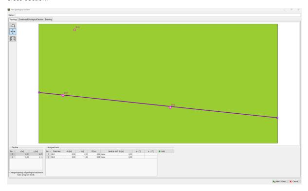
Note: Geological sections are a basic element when creating a 3D subsoil model. Here you can draw your idea of layers. The 3D model will then respect your assignment. Tests and ground profiles that do not pass through the section can be displayed as well.
