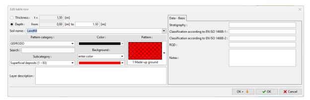
When inputting the second and third borehole, we can either copy the first borehole and edit the layer thickness or re-enter the borehole and only assign the already entered soils from the catalog.
