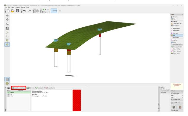
Note: In a real geological survey we can have a large number of soils with minimal differences. For a geotechnical model, it is suitable to merge these soils into a "Geotechnical type" and work with those. The soils (geotechnical types) that we input here will be used not only in a 3D subsoil model but will be transferred to other GEO5 programs too.
