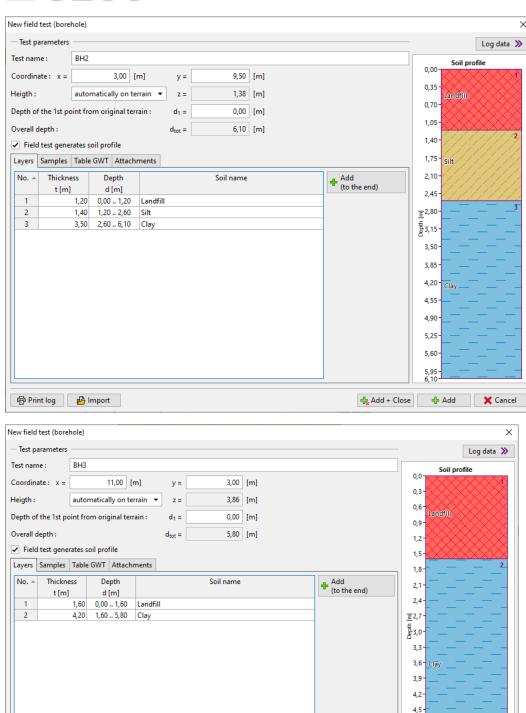
Note: For a real borehole, we usually enter a much larger number of layers and descriptions. We can also enter the information about the water, taken samples, upload photos and other attachments. Description of how to create borehole documentation is in the EM no. 42 – Creation of Field Test Documentation.
