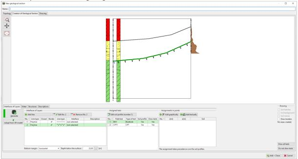
We input assignment points to the areas and assign soils, resp. geotechnical types. If the type is not created already, we can do it now.
