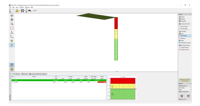
Next, we will interpret the CPT. When the dialog box opens, the program evaluates the CPT test by the Robertson method and will design the soil layers.
