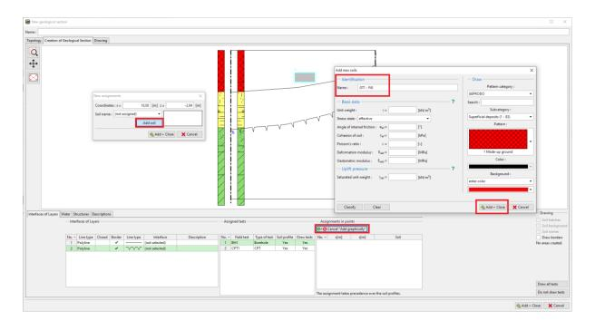
Using "Generate" button we generate area of fill.
