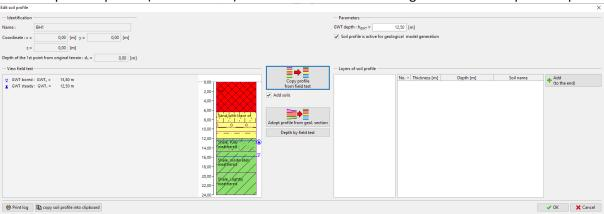
Using "Adopt profile from geol. section" button all data from geological section are transferred into the soil profile.
