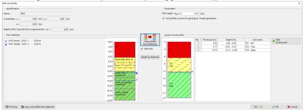
We will repeat the process for the CPT as well. It can be done to the depth of the model (below) or only to the depth of the field test.
