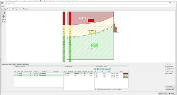
We will open soil profile (borehole BH1) and edit it. We can see dialog window for soil profile input.
