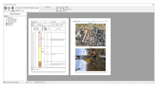
For further modifications of the entered data and for printing the template, we will want to use our standard template. The imported boreholes have a template called "Outside Template - Boreholes". So, we will convert them to our standard template.
