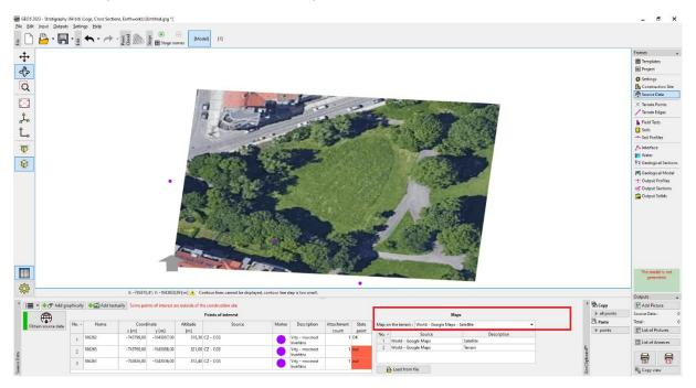
With the "Add graphically" button, we can enter additional points of interest to simplify the survey. For example, assumed positions of wells, landmarks, locations of leveling marks, pipelines, masts, etc.
