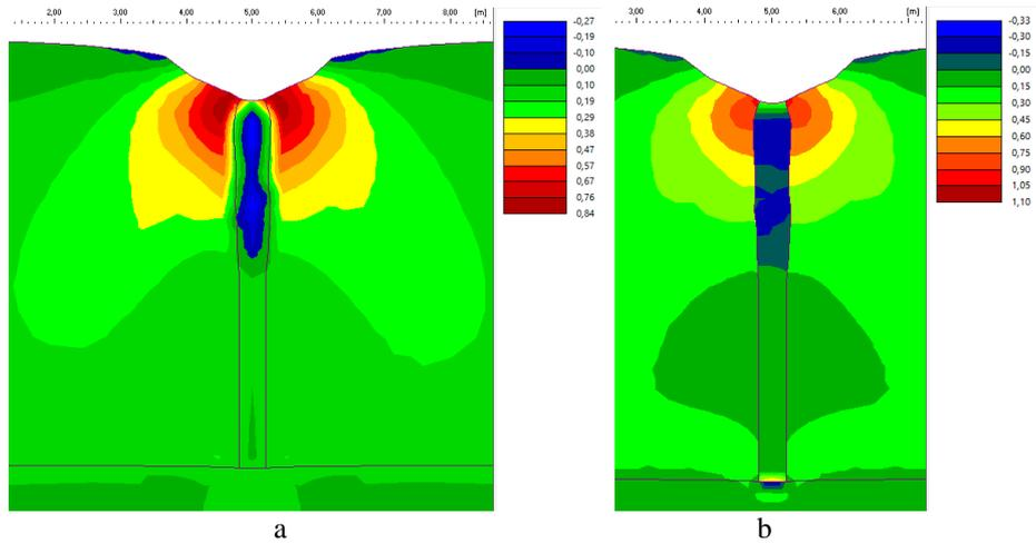
**Fig. 7.** Volumetric Strain Diagram  $\epsilon_v$  [%]: a – unconfined crushed stone column; b – crushed stone column confined with geogrid
