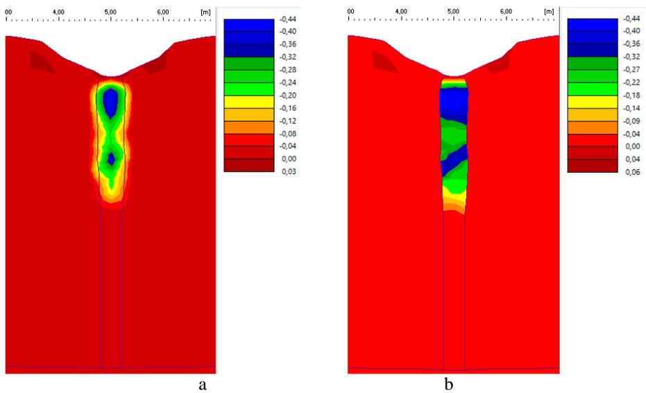
**Fig. 8.** Plastic Volumetric Strain Diagram  $\epsilon_{vp}$  [%]: a – unconfined crushed stone column; b – crushed stone column confined with geogrid
