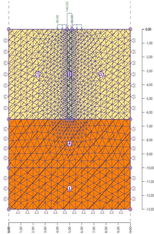
**Fig. 2.** Discretization of the Calculation Domain and the Crushed Stone Column, Boundary Conditions, and External Pressure Applied to the Column and Surrounding Soil
