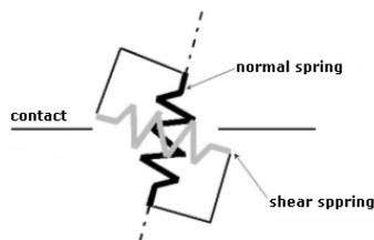
**Fig. 3.** Contact Element Scheme with Visualization of Elastic Stiffnesses [12]
