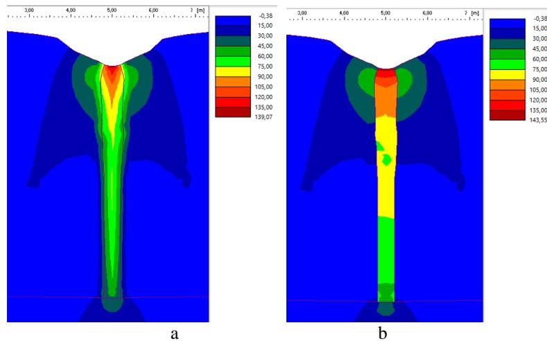
**Fig. 5.** Stress diagram  $\sigma_z$  [kPa]: a – unconfined crushed stone column; b – crushed stone column confined with geogrid
