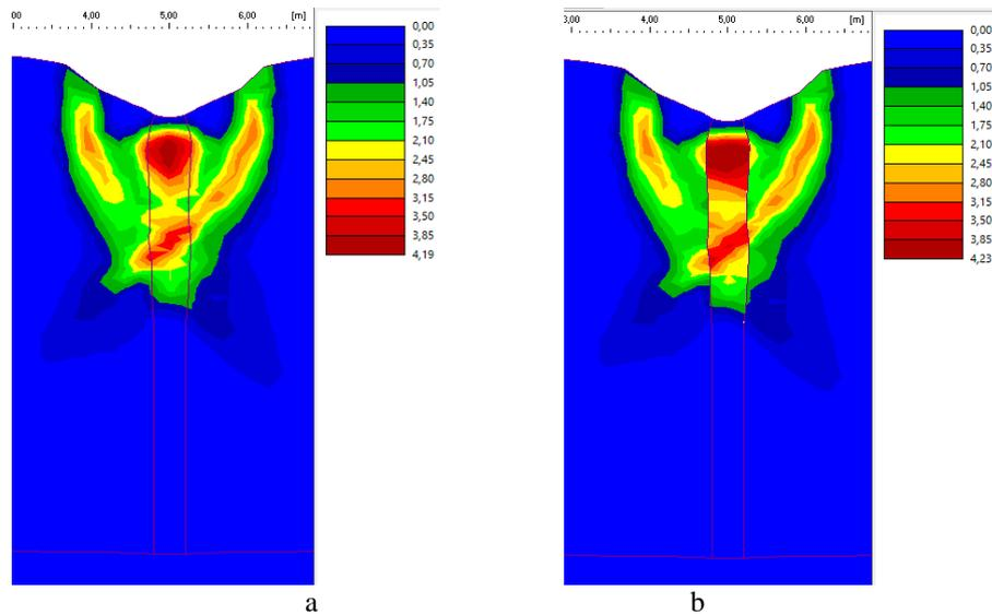
**Fig. 9.** Equivalent Plastic Strain Deviator Diagram  $E_{dpl}$  [%]: a – unconfined crushed stone column; b – crushed stone column confined with geogrid
