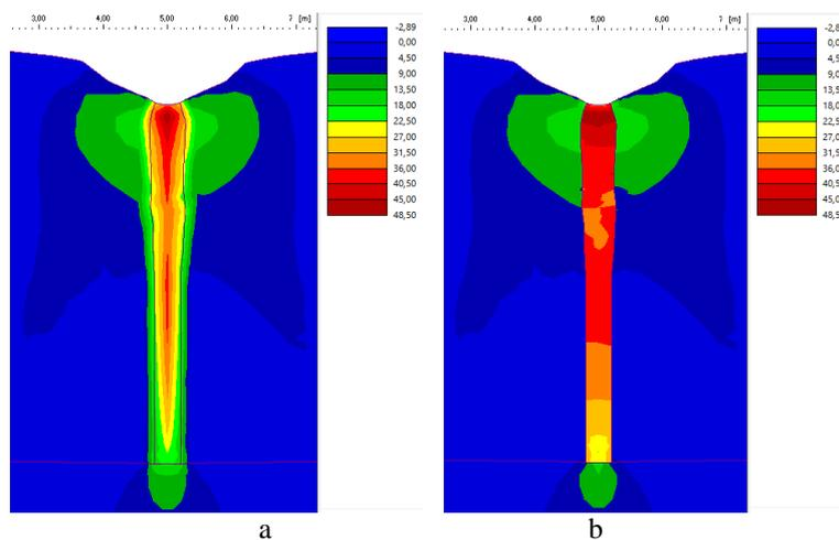
**Fig. 6.** Equivalent Stress Deviator Diagram  $J$  [kPa]: a – unconfined crushed stone column; b – crushed stone column confined with geogrid
