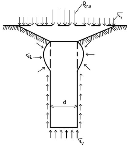
**Fig. 1.** The mechanism of lateral swelling failure of the granular material column. [5]
