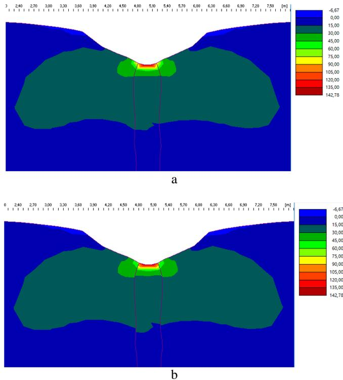
**Fig. 4.** Stress diagram  $\sigma_x$  [kPa]: a – unconfined crushed stone column; b – crushed stone column confined with geogrid
