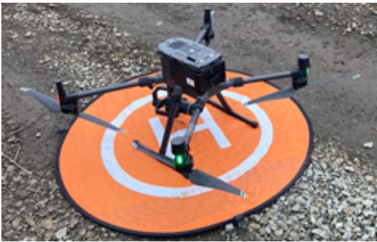
FIGURE 2. DJI M300 RTK drone with camera for photogrammetric measurements.
