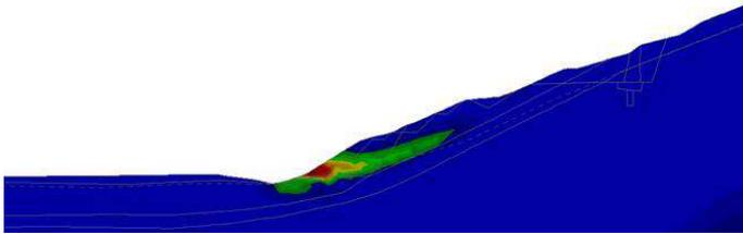
Figure 8. Primary stress state with identified landslide
