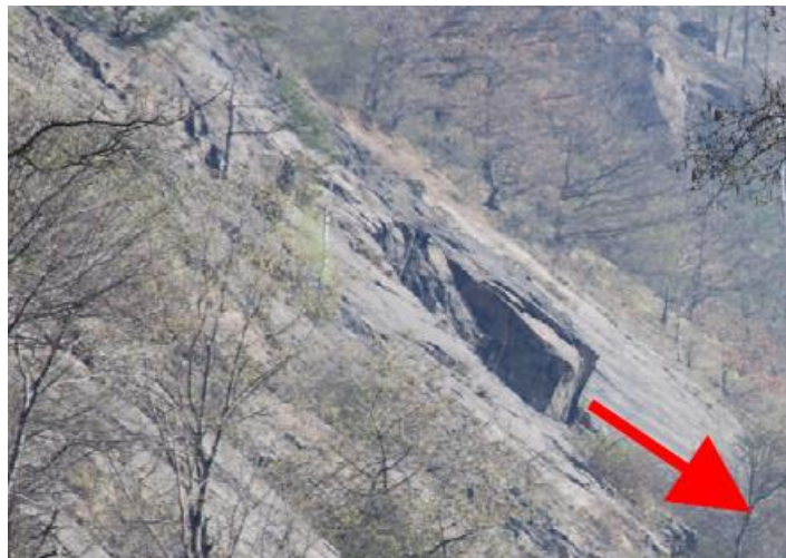
Rock-block with a translation movement presumption (photo Vaniček 2009)
